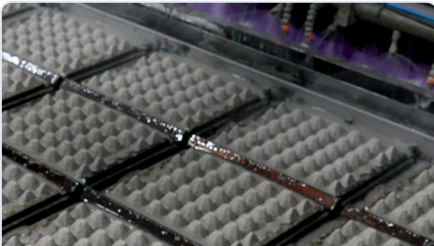
01. Formation Stage: Pulp slurry drawn onto precision suction molds with water spray wash.
