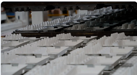
02. After Drying Stage: Cartons exiting high-pressure heated dies with a smooth, low-dust, retail-ready finish.
