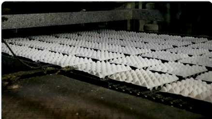
02. Drying Tunnel: Formed trays traveling through multi-zone hot-air drying chamber.
